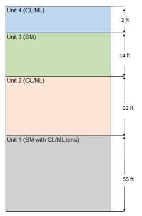
Figure 2 Subsurface Stratigraphy
